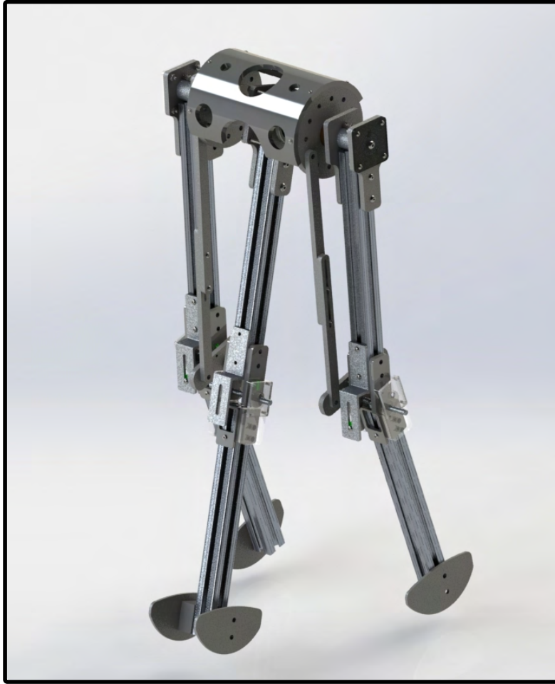
Figure 2.2: A three link physical passive dynamic walker example with rounded feet.
