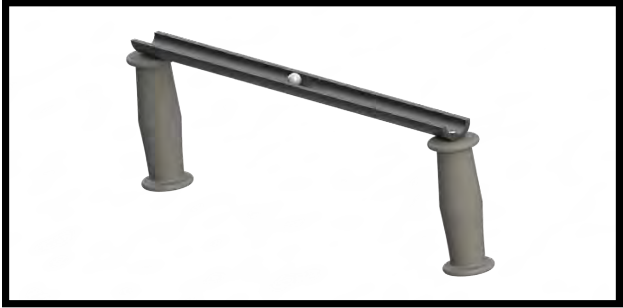
Figure 4.2: Illustration of the distraction device that was used in the experiment. Participants were asked to balance the ball in the middle of the device while walking for two minute sessions.
